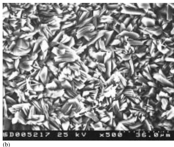
Figure 1 XRD spectra (a) and SEM photograph (b) of electrochemical deposition coating.
